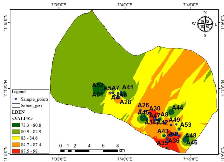
Figure 6. The diurnal  $L_{DEN}$  average noise level mapping for the summation of day time, evening, and night time intervals, respectively.
