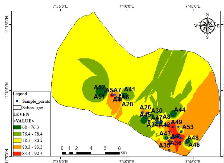
Figure 4. Spatial noise map for the evening interval from 6 PM to 11 PM.
