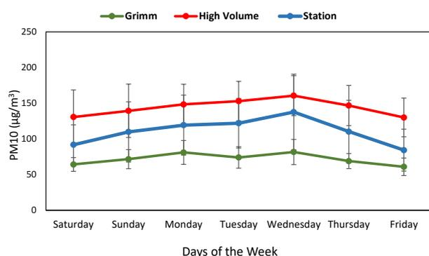
**Figure 3.** Daily variations of  $PM_{10}$  in TB monitor, high-volume sampler, and portable PM monitor
