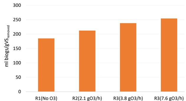
**Figure 8.** The value of biogas production from digesters containing ozonated and non-ozonated samples (15% LL/85% SS)
