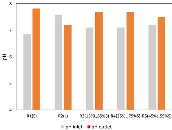
**Figure 4.** Inlet and outlet of pH in digesters containing various ratios of leachate to sludge
