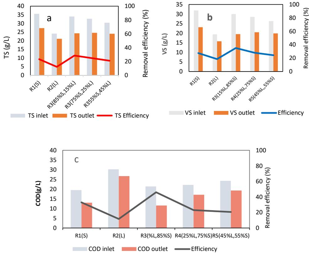
Figure 2. Inlet and outlet concentration and removal efficiency of (a) TS, (b) VS, and (c) COD in digesters containing various ratios of leachate to sludge
