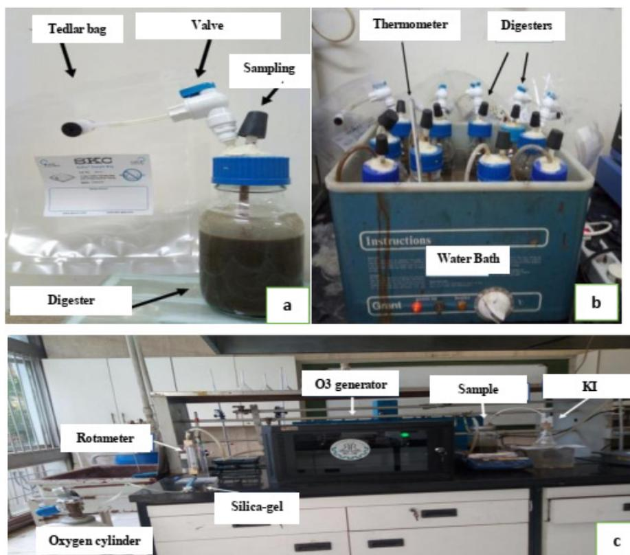
**Figure 1.** Images of anaerobic reactors and ozonation apparatus (a) One of the digesters and its accessories, (b) Digesters in water bath, (c) Ozonation apparatus
