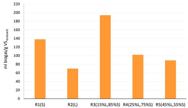
**Figure 5.** The value of biogas production from digesters containing various ratios of leachate to sludge
