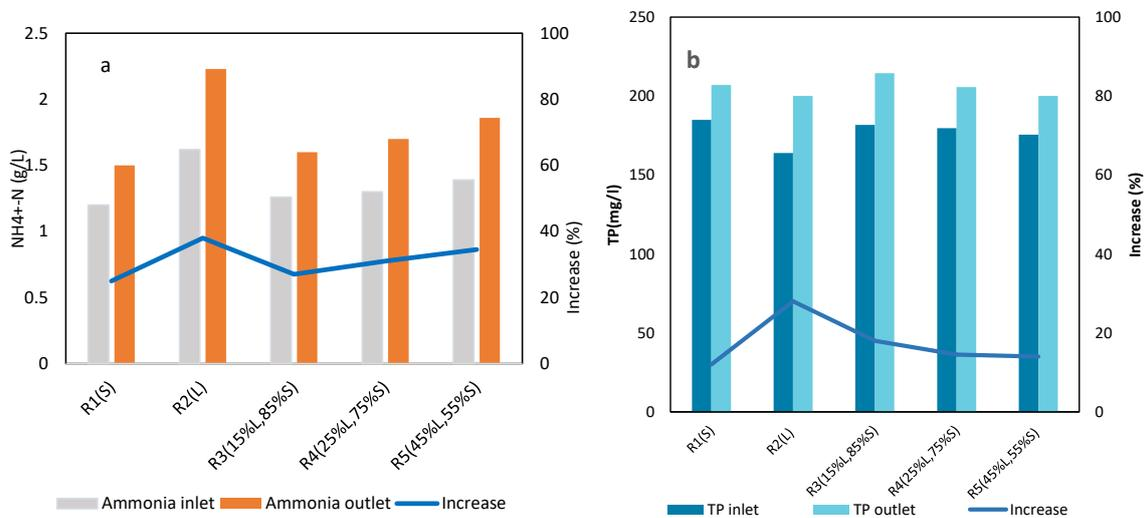
Figure 3. Inlet and outlet concentration and removal efficiency of (a) Ammonia, and (b) Phosphorous in digesters containing various ratios of leachate to sludge
