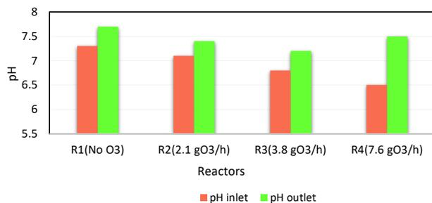
**Figure 7.** The inlet and outlet of pH in digesters containing ozonated and non-ozonated samples (15% LL/85% SS)
