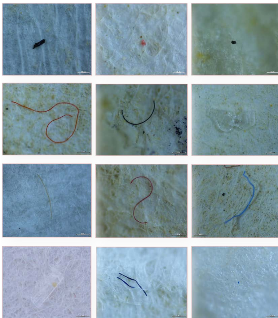
Figure 2. Examples of microplastic particles observed through a microscope include fiber particles, pieces, and films
