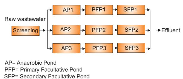
Figure 2. Schematic flow diagram for M1 AWSP
