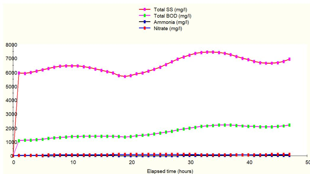
Figure 6. Sludge flow properties in stream 8 with elapsed time.
