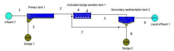
Figure 1. Model design simulation of wastewater treatment plant basic components.
