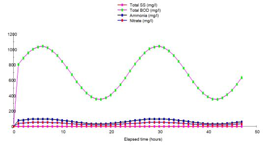
Figure 3. Continuously dynamic flow of wastewater to the treatment plants with pollutant properties.
