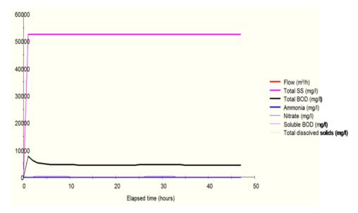
Figure 5. Sludge flow properties through the stream 3 with elapsed time.
