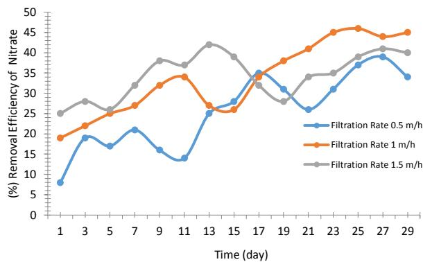
**Figure 1.** Changes of nitrogen removal efficiency at three filtration rates.
