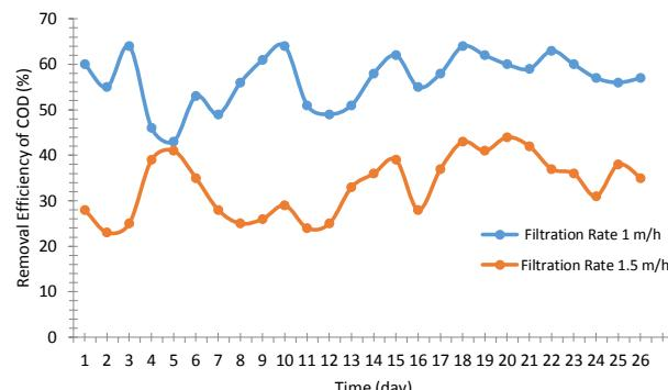
**Figure 4.** Changes of COD removal efficiency at filtration rates of 1 and 1.5 m/h.
