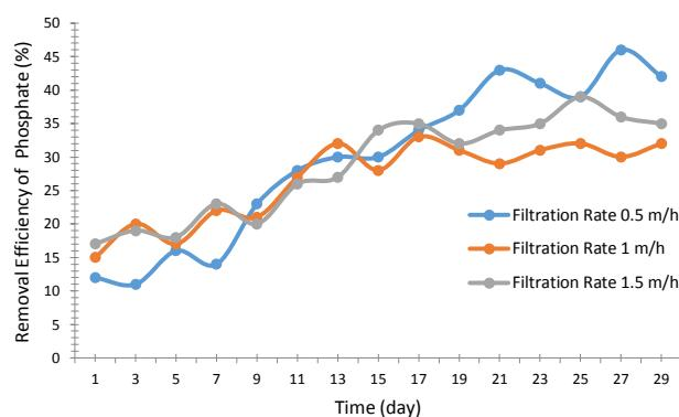
**Figure 2.** Changes of phosphate removal efficiency at three filtration rates.
