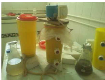
Figure 2. Flow diagram of the anaerobic sequencing batch reactor (ASBR) experimental setup.
