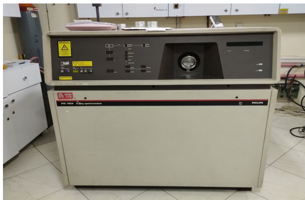
Figure 3. X-ray fluorescence device to extract the chemical structure of the packing materials
