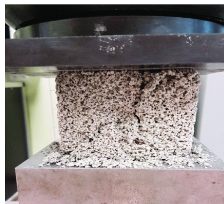
Figure 2. CLC waste used in this study under compressive strength examination
