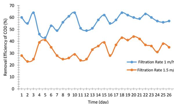
**Figure 4.** Changes of COD removal efficiency at filtration rates of 1 and 1.5 m/h.
