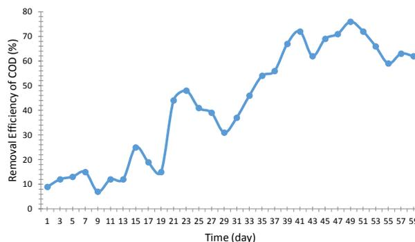
**Figure 3.** Changes of COD removal efficiency at filtration rate of 0.5 m/h.
